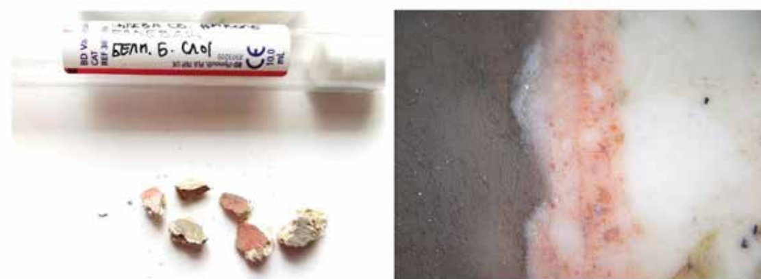
Fig. 20. Sample 3, red or blue painted layer with a white coating. Cross-section of the sample with a magnification of ca 350x (photo by T. Tripković).
