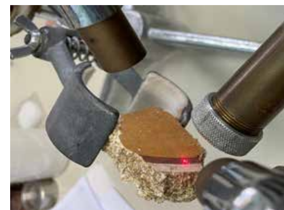
Fig. 5. Detail of an EDXRF spectrometric examination of the dark red pigment on a fragment of a wall painting (Photo by M. Gajić Kvaščev).
