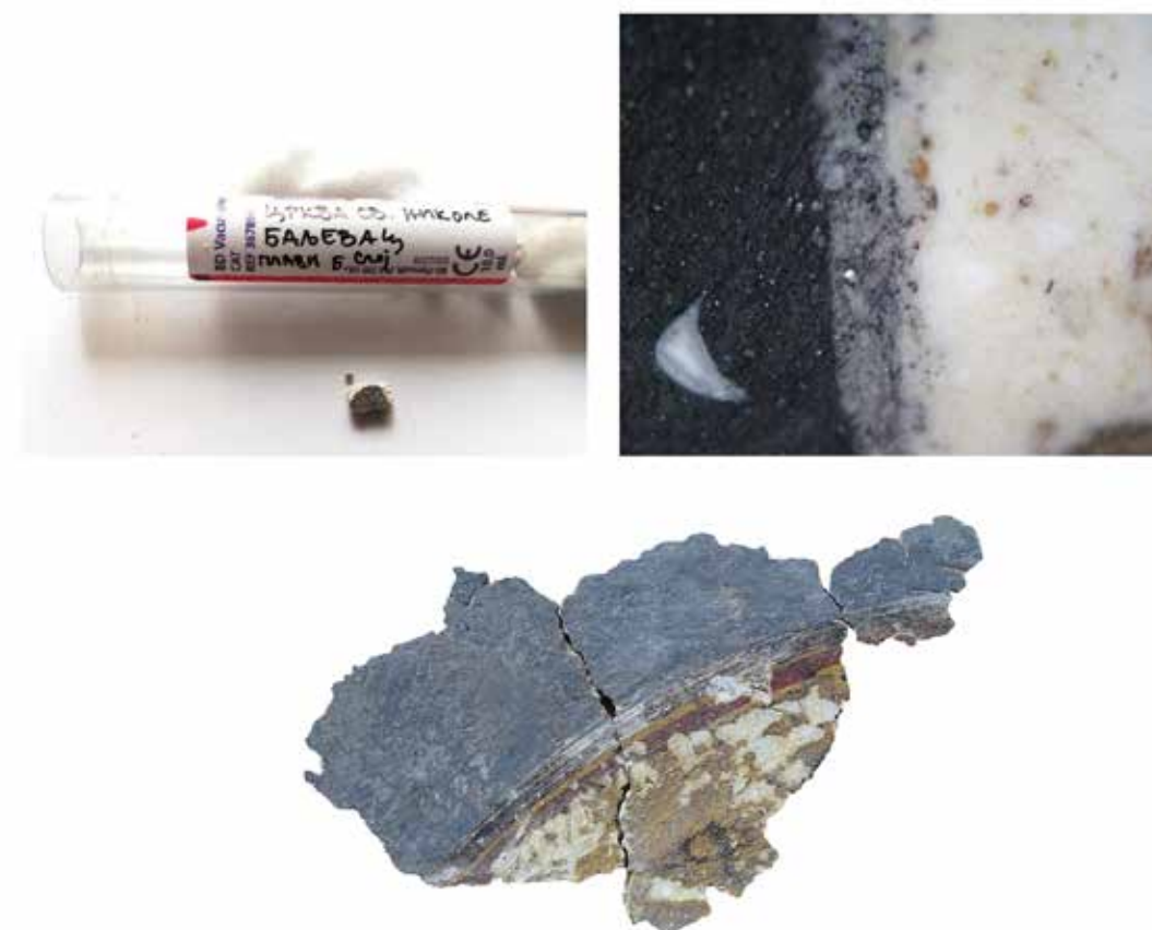
Fig. 21. Sample 4, black. Cross-section of the sample with a magnification of ca 350x (photo by T. Tripković).
