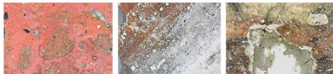
Fig. 4. Appearance of the painted layers of fragments with a magnification of ca 50x (Photo by K. Ponjavić).
