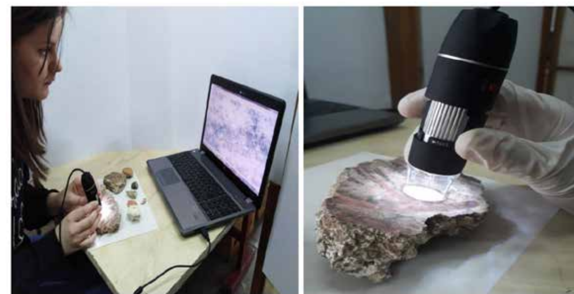
Fig. 3. Examination of the surface of the painted layers of fragments with a USB microscope (Photo by K. Ponjavić).
