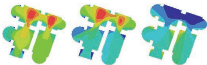
Fig. 9. Graph of Connectivity, Visual Integration, and Visual Mean Shortest Path of the first phase of the Roman bath in Timacum Minus
