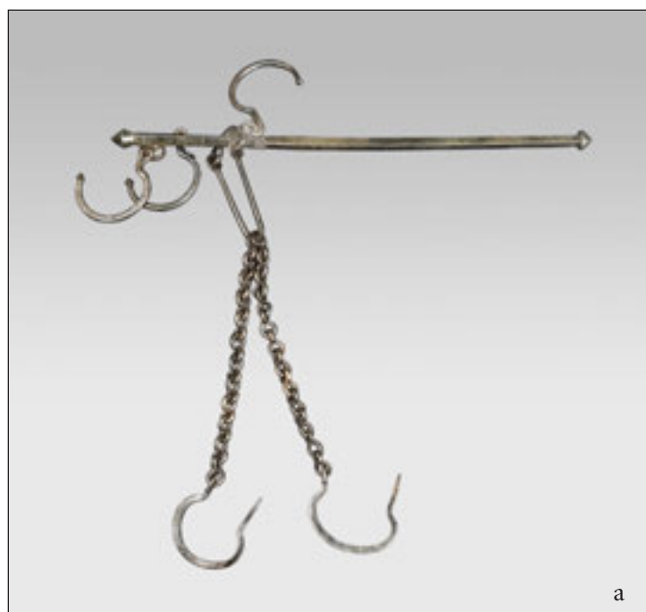
FIGURE 162. Parts of steelyard and weight for weighing grain and other goods (a), with inscription Ρουστικλου (b), 6 th century
