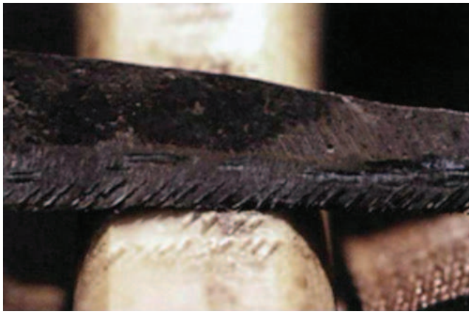
Fig. 6: Detail of the process of cutting teeth into a sickle. It is clearly visible how each tooth corresponds to a V-shaped indentation on the bone anvil, after Esteban-Nadal & Carbonell Roure (2004: fig. 13).
