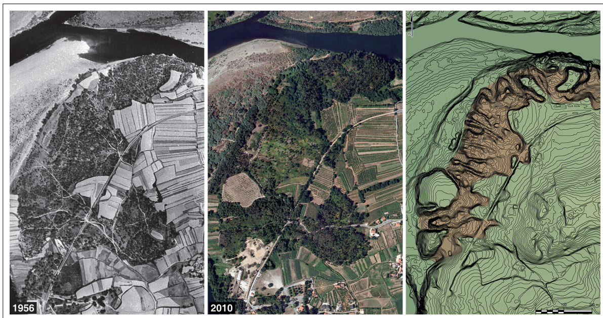
Figure 6. Morphological analysis of the Roman gold mining exploitations of Cortes (Monção, Portugal). The combined analysis of aerial photographs of the “American flight” and the ALS-derived topography shows mining workings carried out by the so-called method of “series of convergent furrows”. © Elaborated by EST-AP, CSIC, from the USAF “American flight” (series B, 1956), the IGN PNOA flight (2010) and an ALS-derived terrain model (contour line interval = 0,5 m).
