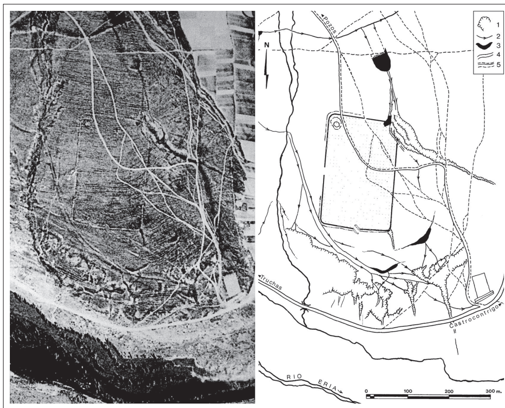
Figure 2. Photo-interpretation of the mining exploitations and Roman fort of Valdemedina (Truchas, León). Legend: 1: mining exploitations; 2: network of Roman water canals for the supply of water to the mining exploitations; 3: water reservoirs; 4: modern main road; 5: modern secondary road (cfr. Fernández et al. 2015, figure 10, where the isolated use of ALS makes it impossible to detect many of these structures). Elaborated by EST-AP, CSIC.
