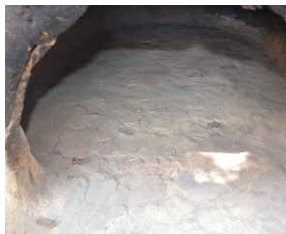
Fig. 9 – Experimental oven from 2012. after several years of usage (floor)
