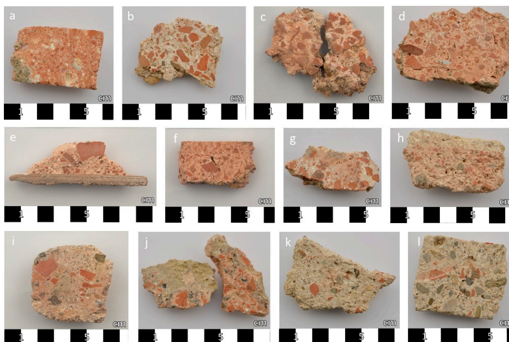
Figure 2. “Brick” mortars from Viminacium (dating from the 2nd to the 6th century): (a) principium floor; (b) city baths floor; (c) city baths plaster; (d) city baths floor; (e) city baths plaster; (f) city baths plaster; (g) city baths plaster; (h) tomb plaster; (i) sarcophagus base; (j) villa floor; (k) villa bedding mortar; (l) early Byzantine rampart bedding mortar. Photo documentation of the MoDeCo2000 project.
