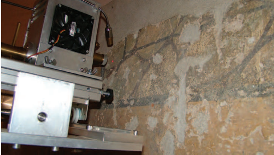
Fig.4. A detail of the analytical process of identifying the green pigment, carried out by applying the pEDXRF technique
