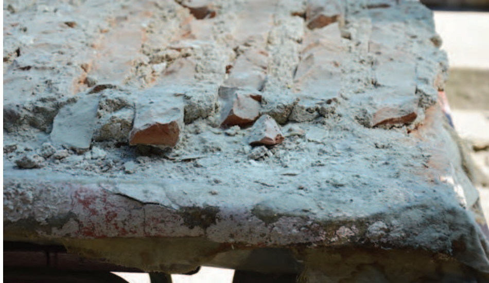
Fig.2. The back of the wall painting before the works, showing the overhang of the wall painting on the edge of the support.
