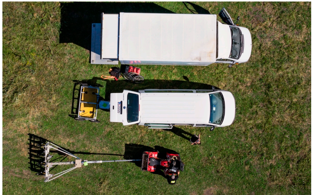
Figure 5. Aerial photograph of the 6-channel SPIDAR GPR system (center) and the magnetometer system (bottom) with their corresponding towing vehicles on site, photographed from the UAS. Photo: Geert Verhoeven.
