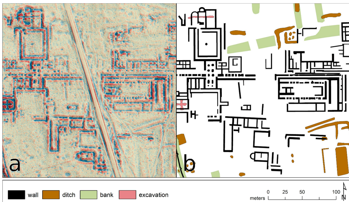
Figure 12. (a) Detail of a fused DSM visualization: a simple local relief model (circular kernel with 40 cells radius, (-0.15\text{ m}, 0.15\text{ m}) clip, blue-yellow-red colour map) merged with a multidirectional hillshade ( 35^\circ solar elevation, vertical exaggeration factor of 3) using two iterations of the “hard light” blending mode with varying opacity levels. The contrast of both source layers was slightly altered before the initial blending. (b) Corresponding archaeological interpretation.
