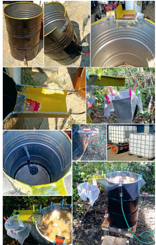
Fig. 28. Stages in the construction of a flotation tank for Svinjarička Čuka (Photos: D. Filipović).
