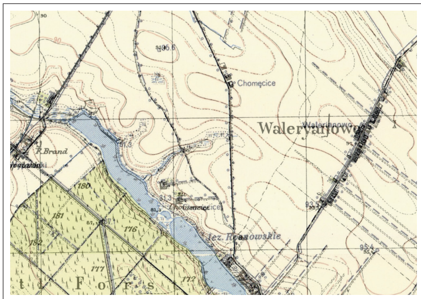
Figure 13. Fragment of mapa powiatowa against a background of a German Mestischblatt . This example shows a compilation method in practice and (in) accuracy in depicting contours which was probably caused by poor copying. ©Topographic Unit, General Staff of the Polish Army.
