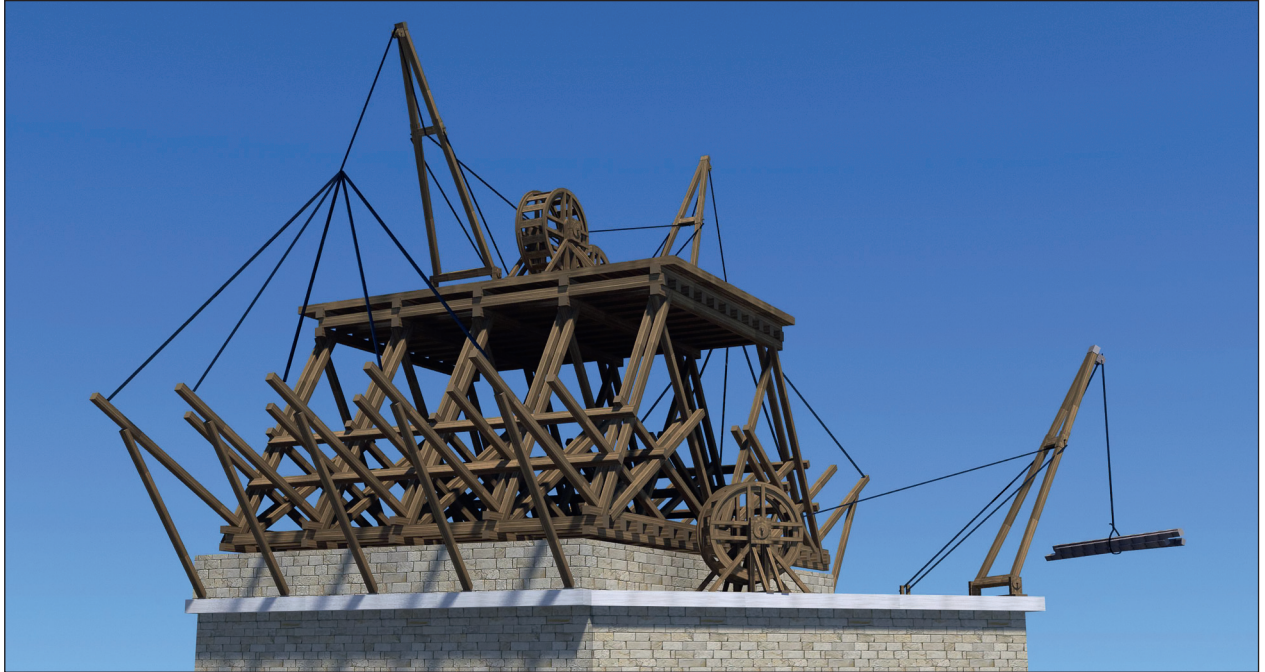
Figure 5. Position of the machinery for vertical load lifting in the process of building the wooden structure (reconstruction by the author, 3D model V. Milošević)
