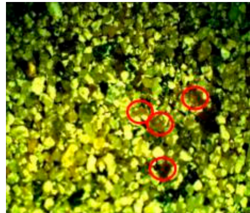
Fraction 250–125 \mu\text{m} Crushed brick particles marked; magnification \times 20
